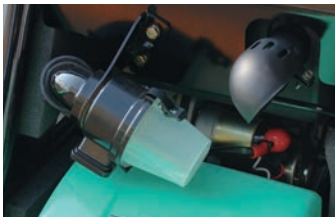
Mikasa cyclone series(MVH-206 ~ 508 diesel engine) Cyclone pre-cleaner increase filterability dramatically! Most suitable for harsh environment
