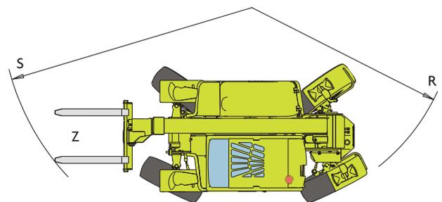
The engine is mounted to the right side of the chassis, ensuring safe, easy access and maintenance from ground level.
